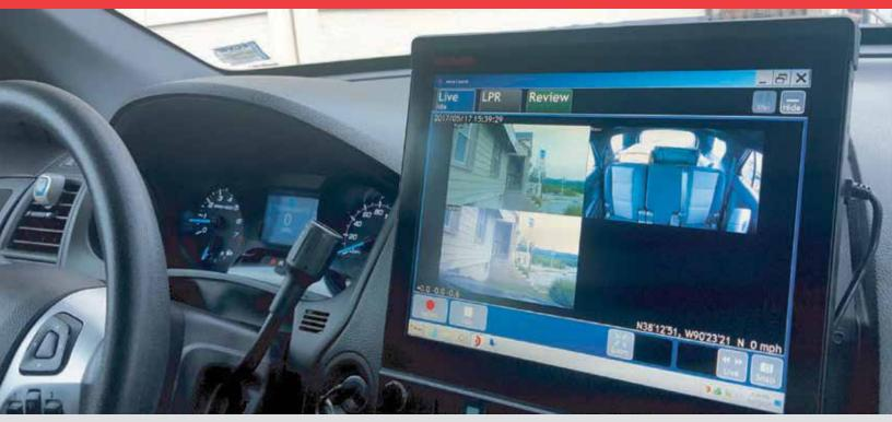
All M series computers are designed for harsh vehicular environments and extreme temperature conditions. The modular 3-piece design allows for a variety of airbag-compliant mounting options and cost-effective upgrades. The M8 is backward compatible with all generations of Data911 M series mobile computers.
