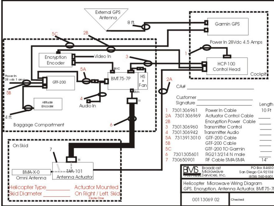
The GCA-4 antenna system uses GPS to steer the antenna and point at the receive site. The operator needs only to input the coordinates of the receive site for the antenna to point. Significantly extended ranges are attainable by this system, but, as can be seen from the block diagram above, the system is more complex and expensive than an omni directional system.
