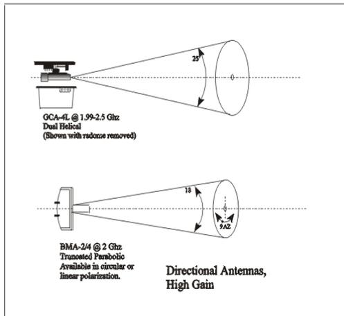
High Gain Directional antennas have a focused beam width and a conical coverage area. The higher the gain, the more focused the beam width becomes. Because of the conical antenna pattern, high gain antennas need to be pointed at the transmit or receive site. This is typically a simple issue until one or both of the sites are moving, as in the case of airborne microwave downlinks.
