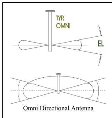
The most common omni antenna, the dipole antenna, is often referred to simply as an Omni antenna. The dipole antenna is shaped like a stick or broom handle. Versions of dipole antennas appear on cellular phones, two-way radios, and car radio systems. The 360 degree pattern from an Omni antenna is shaped like a donut.
