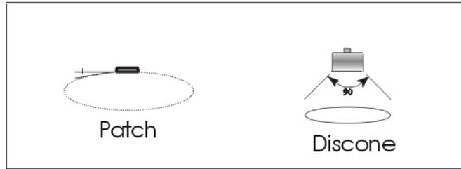
*Patch Antennas and Discone Antennas are omni antennas with a different pattern.*
