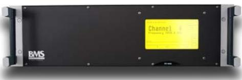
Designed for use at ENG central receive sites, the DR2000 and DR6000 both employ a dual IF/RF AGC control with 70 dB dynamic range and will typically produce a C/N improvement of 6-9 dB for a 2 way diversity system over a standard single channel receiver.
