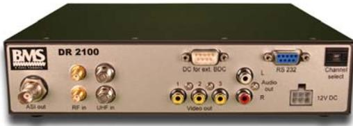
The DR2100 2-way diversity receiver is DC powered and compact in size. It is fully self-contained with built in down converters making it ideal for use on portable links and for wireless camera reception.
